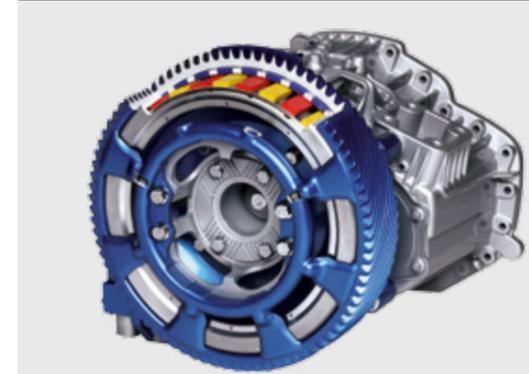
This low-wear and maintenance-free auxiliary braking system allows additional braking power of up to 181 kW in conjunction with braking torque of 650 Nm.
