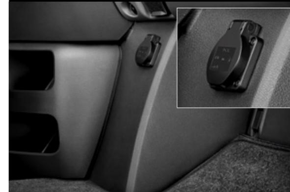
Converts 24 V direct current into 230 V alternating current, protected against overload and short circuit. The inverter allows you to connect a variety of electrical consumers to your on-board power supply, from your laptop to your shaver. Output up to 350 W.
