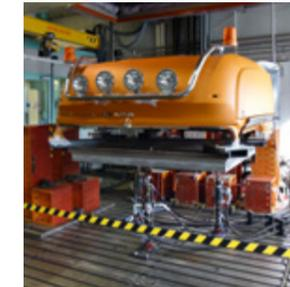
The hydropulse test stand simulates potholes and poor road conditions.
