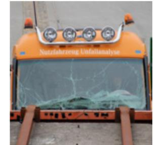
Bending and breaking: roof-mounted headlamp holder in a crash test.
