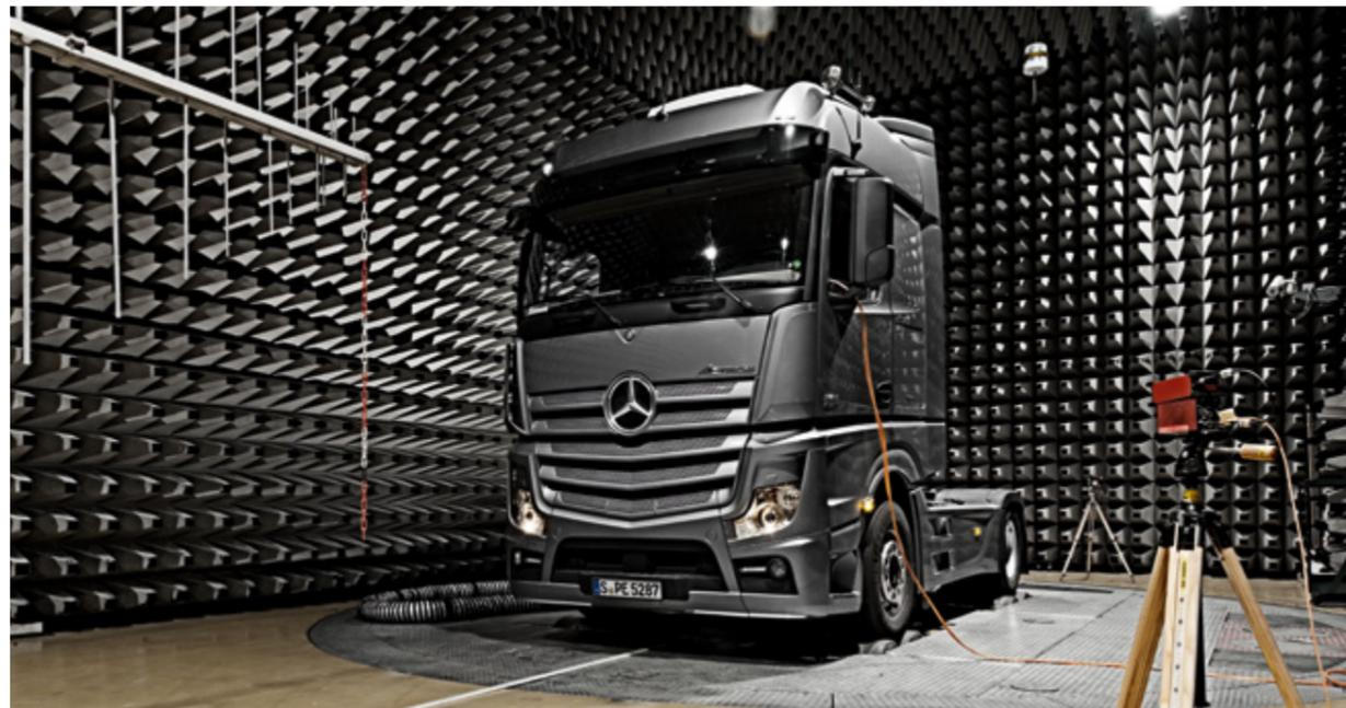
EMC testing in a hall specially shielded against external electromagnetic interference.
